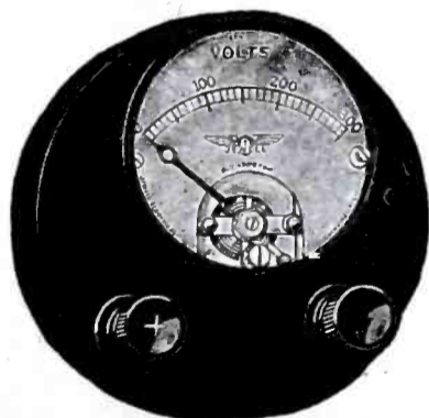
No. 139—A small high resistance voltmeter of the D'Arsonval type suitable for use by the individual in checking and adjusting B-eliminator voltages. 0-300 volt scale.
